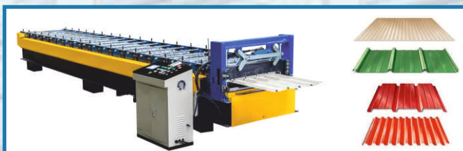
On Site Forming Machine
